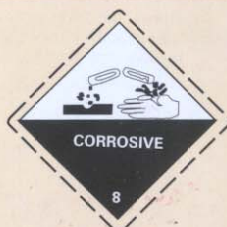
Corrosives Symbol (liquids spilling from two glass vessels and attacking a hand and a metal) : black Background : upper half white lower half black with white border
