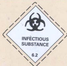
Division 6.2 Infectious substances Symbol (three crescents superimposed on a circle) and Inscription : black Background : white
