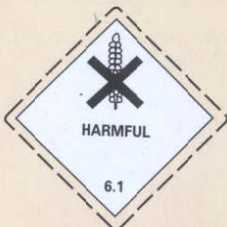
Division 6.1 Poisonous (toxic) substances Stow away from Food Stuffs Symbol : black, Background : white
